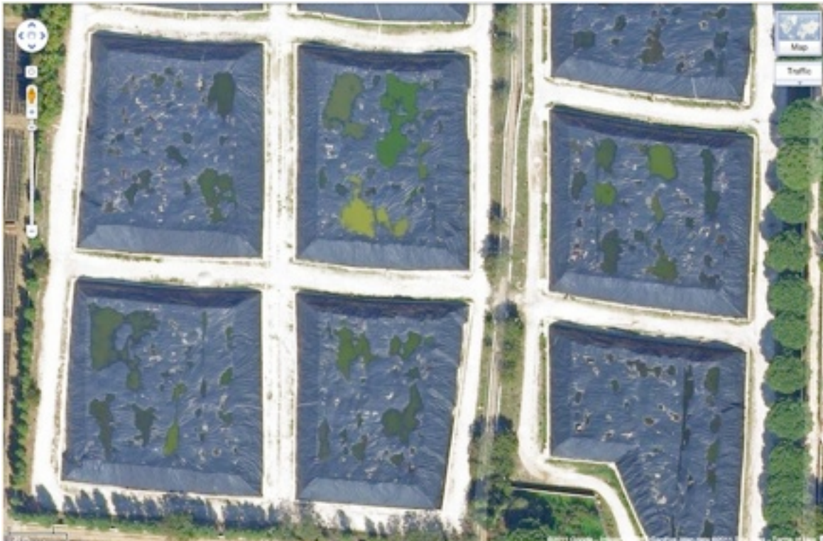
Evidence 15: Ponte Riccio Landfill - Water accumulations on the plastic insulations, Giugliano - Credits: Google Inc.
